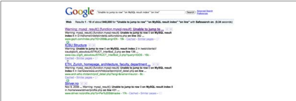
Figure 1-4. Execution of an SQL injection dork
