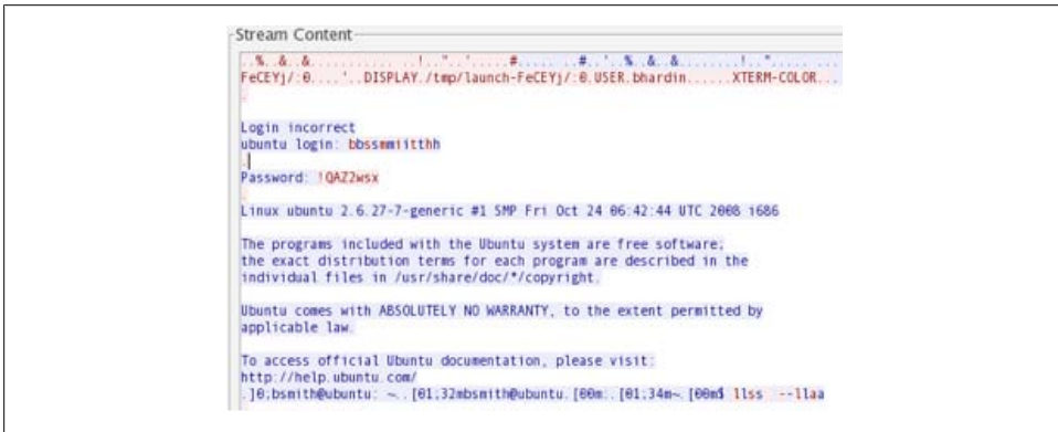
Figure 3-1. Captured Telnet data on the attacker's machine
